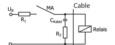
Contact protection with resistors for limiting current
