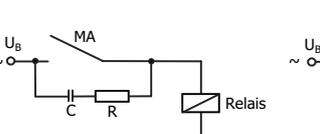
Suppression of voltage peaks with an RC element
