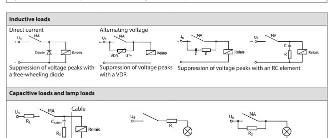
Contact protection with resistors for limiting current
