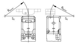
$R_{\text{Amin}}$  and  $R_{\text{Bmin}}$  depend on the actuator. Applies accordingly also to lateral retraction directions.
