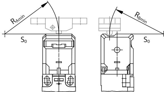
$R_{Amin}$  and  $R_{Bmin}$  depend on the actuator.
