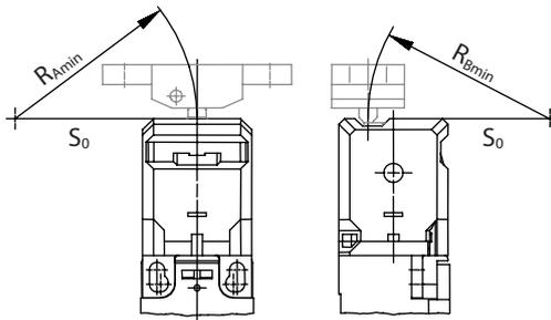
$R_{Amin}$  and  $R_{Bmin}$  depend on the actuator.
