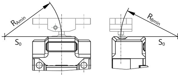
$R_{Amin}$  and  $R_{Bmin}$  depend on the actuator.
