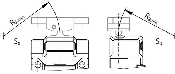
$R_{Amin}$  and  $R_{Bmin}$  depend on the actuator.
