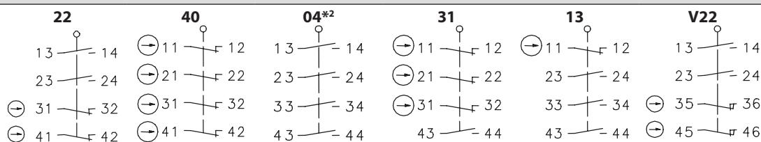
**Operating diagram when using the actuator on an IN73/MN78 with 4 switching contacts...**
