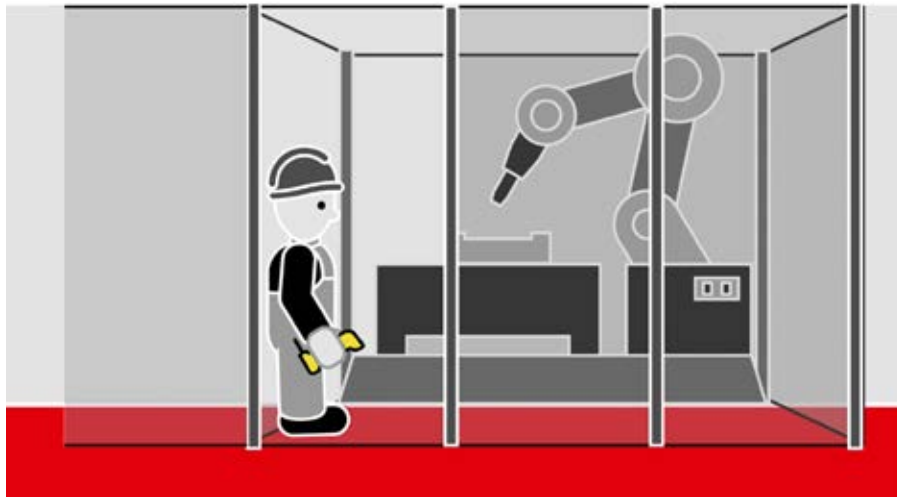
Teaching a robot function through a manually operated enabling switch
