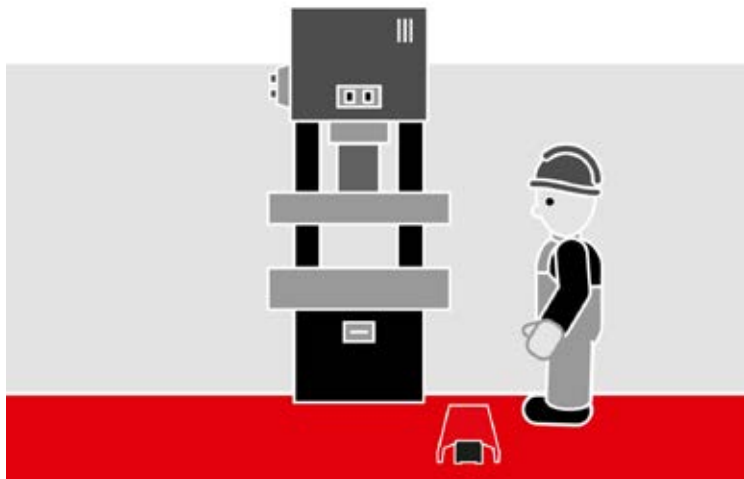
Enabling foot switch for inching operation on a press
