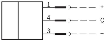
C = Control-Input. The emitter will be turned off when „Control“ and „-“ get connected (system test).
