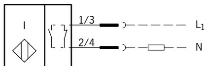
The normally-open or normally-closed function can be selected via an integrated switch.
