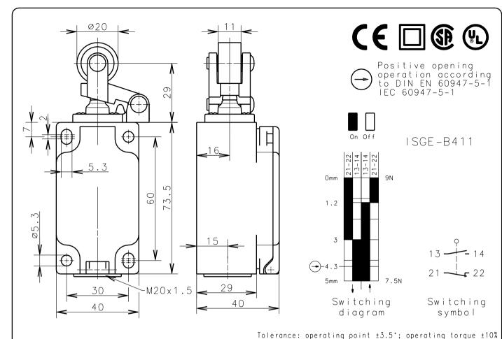
Mechanical features Thermoplast, glass fibre reinforced Enclosure: Cover: Thermoplast, glass fibre reinforced Actuator: Lever (Zn-die cast), Roller (thermoplast) Ambient air temperature: -30°C up to +80°C Contact type: 1 NC-contact, 1 NO-contact (Zb)
